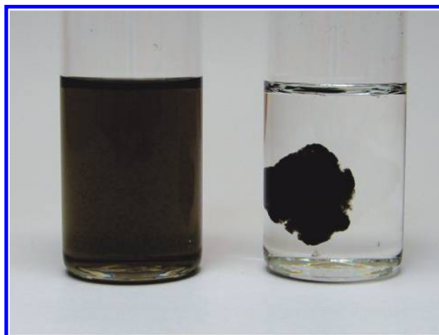
Figure 1. The dispersion on the left was ultrasonicated for 2 h without being cooled by an ice bath. The sample on the right was ultrasonicated for 2 h with an oxygen sparge and kept at \sim 20 °C by an ice bath.
